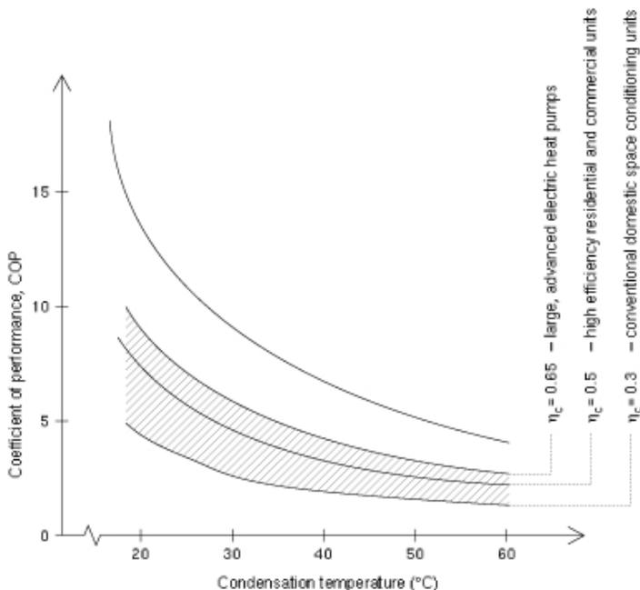
Figure 1 shows the COP for an ideal heat pump as a function of temperature lift, where the temperature of the heat source is 0°C. Also shown is the range of actual COPs for various types and sizes of real heat pumps at different temperature lifts.
