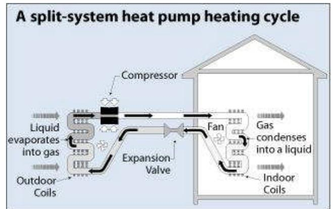
near the compressor, can change the direction of the refrigerant flow for cooling as well as for defrosting the outdoor coils in winter.
